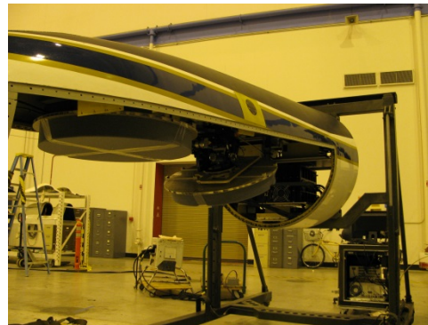
Figure 1. EXRAD measurement concept. Conical or cross-track scanning beam and nadir beam.
