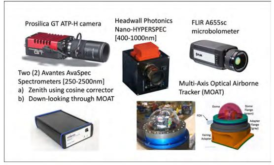
Figure 36. HYPPOS aircraft instrumentation.
