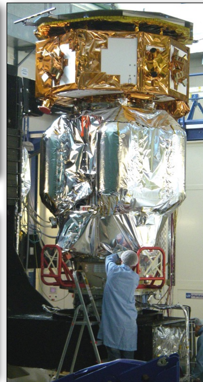
Transfer Orbit Thermal Test
