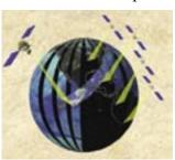
The Global Precipitation Mission (GPM) is designed with a core satellite flying with a constellation of satellites to provide accurate global estimates of horizontal and vertical structure of rainfall and microphysics elements.
