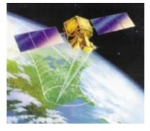
Global Wind Explorer – A mission concept to directly observe the dynamics of the atmospheres using a Doppler lidar to profile wind in the troposphere and stratosphere.
