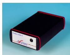
Figure 4.4: A small inexpensive spectrometer system measuring UV and VIS light from 270–525 nm in 0.5 nm steps. The system consists of an optical head, containing internal filter wheels, mounted on a Sun-sky tracker. The optical head as shown is then mounted on a tripod. The optical head is coupled to the small spectrometer by a 10-m fiber optic cable. The entire spectrometer is maintained at a constant temperature of about 20°C within 1°, using thermoelectric heating and cooling of an insulated waterproof box.
