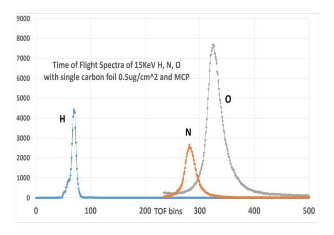
Time of Flight mass spectra of 15keV H, N, O beam from the lab prototype of a 0.5ug/cm^2 carbon foil - MCP TOF sensor. Separation of N,O demonstrates M/dM ~12.
